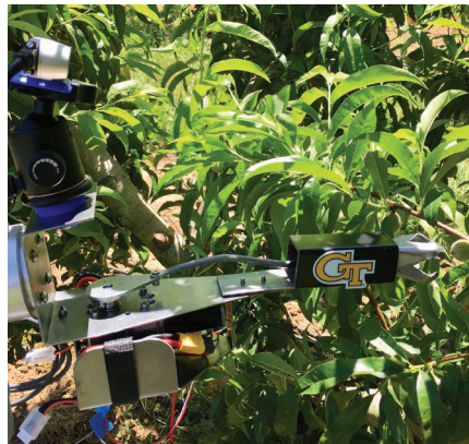
A close-up of the end effector device that grabs and removes peachlets.
