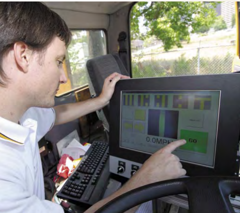
Pavement marker placement is controlled by an in-cab system.
