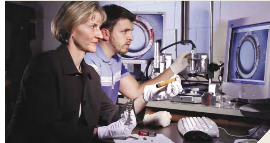
Researchers examine textile machinery components damaged by chlorine.
