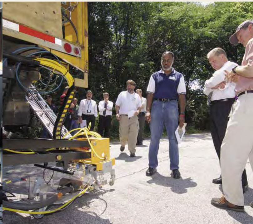
Researchers examine pavement marker placement system.
